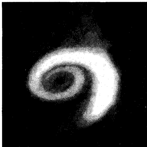
Fig. 8 Laser sheet smoke visualization of tip vortex at X/C = 1.67 downstream of the forward-swept vane.
