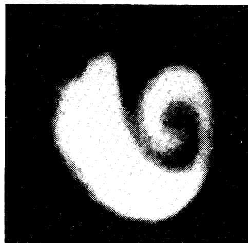
Fig. 7 Laser sheet smoke visualization of tip vortex at X/C = 1.0 downstream of the unswept vane.
